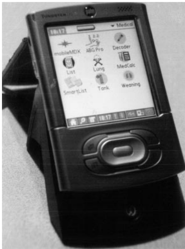
Fig. 6. Palm Model Tungsten T-2 personal digital assistant in its cradle. Pressing the HotSync button downloads the clinical and billing data to the hospital's network server database.
