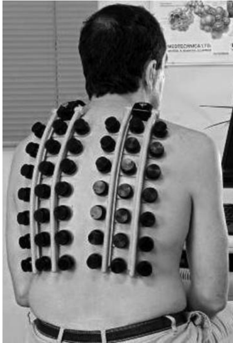
Fig. 1. Placement of the sensor array. Low-pressure vacuum attaches the sensors to the skin.
