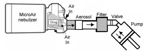
Fig. 1. Test setup.
