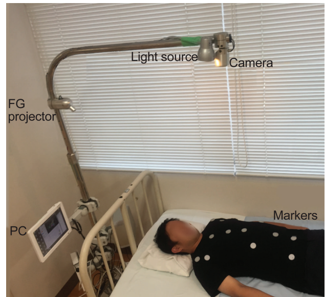
Fig. 1. Experimental setup for RMET measurement. RMET = Respiratory Movement Evaluation Tool, PC = personal computer, FG = fiber grating.
