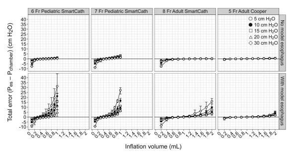
Fig. 2. The mean and range (error bars) for total error of the esophageal balloon catheters as a function of esophageal balloon inflation volume, and set chamber pressure ( $P_{chamber}$  5, 10, 15, 20, or 30 cm  $H_2O$ ) stratified by the presence and absence of a model esophagus, and catheter type.
