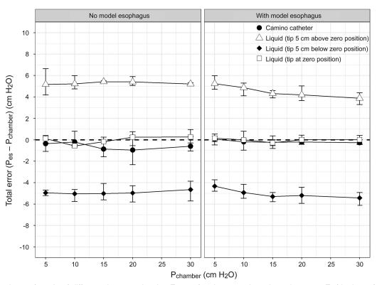
Fig. 5. Mean and range (error bars) difference between chamber ( $P_{chamber}$ ) and measured esophageal pressure ( $P_{es}$ ) is shown for the Camino catheter (micro-tip transducer) and the liquid-filled catheter (8 Fr CORFLO) when the liquid-filled catheter tip is level with the transducer and both 5 cm above and below the transducer, stratified by the presence and absence of a model esophagus.
