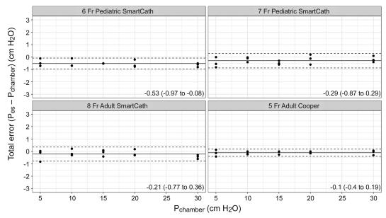
Fig. 4. Mean total error and precision (95% CI) is shown with Bland-Altman plots when using a model esophagus and an esophageal balloon inflation volume that corresponds with the optimal filling volume for each testing condition. Results are stratified by catheter type.
