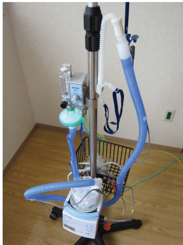
Fig. 2. Experimental setup for Optiflow. An exclusive circuit and a filter for noise reduction were attached on the total flow out-take side of Optiflow using the medical gas outlet for oxygen and air as the driving source. The tip of the nasal cannula hung freely.
