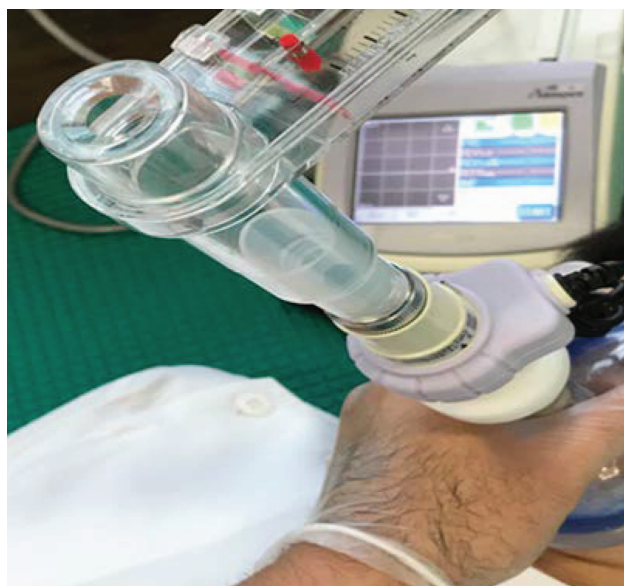
Fig. 1. Connection of the spirometer (Minato) and peak flow meter (Philips Respironics).
