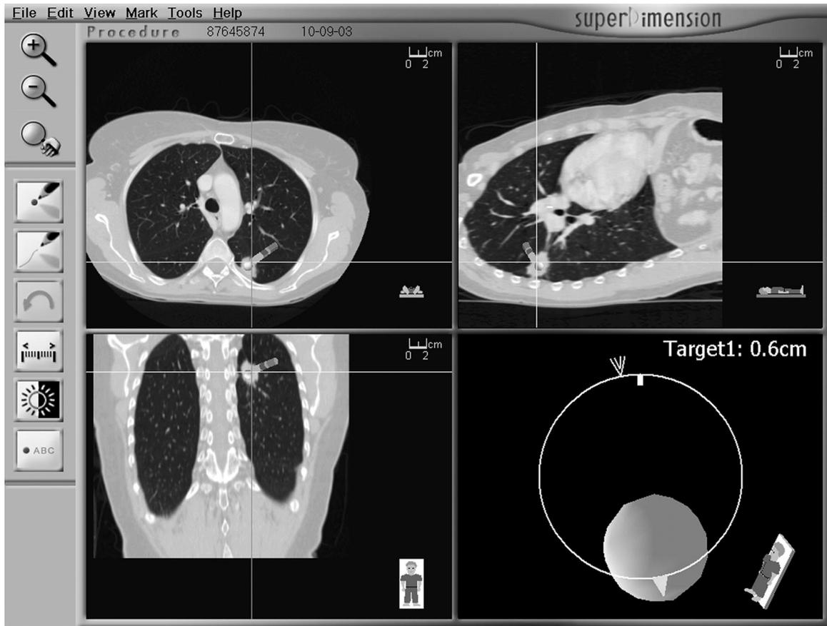
Fig. 2. Computerized sensing of bronchoscope location. Pictured are 3 planes of a computed tomography image of a patient with a lesion in the left upper lobe. The patient lies on a platform that contains sensors that detect the position of the bronchoscope tip (striped rod). That information is superimposed on the CT image, showing the bronchoscope's position with respect to the lesion. (Courtesy of superDimension GmbH, Düsseldorf, Germany.)
