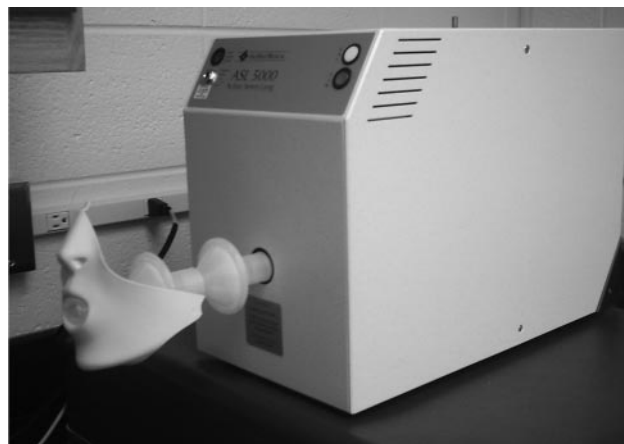
Fig. 1. Configuration of equipment for simulation of pediatric breathing and nebulized albuterol delivered via face mask, with the mask at 0 cm, 1 cm, and 2 cm from the chin of the mannequin face.
