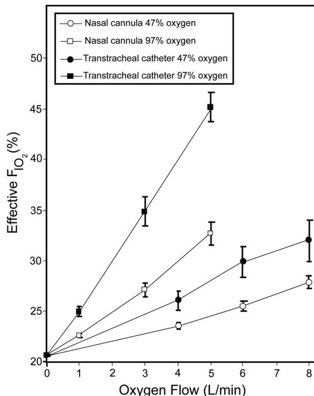
Fig. 4. Effective fraction of inspired oxygen (effective  $F_{IO_2}$ ) versus oxygen flow rate with 2 different oxygen supply systems (membrane separator and molecular sieve) and 2 different oxygen delivery systems (nasal cannula and transtracheal catheter). Data are expressed as mean ± SEM.
