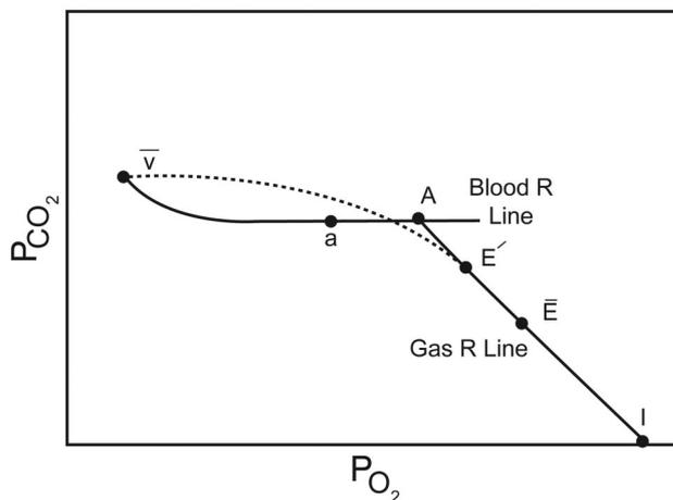
Fig. 2. The  $O_2$ - $CO_2$  diagram of Rahn and Fenn.<sup>6</sup> To find the effective fraction of inspired oxygen (effective  $F_{IO_2}$ ) we extrapolate along the gas line to the intersection on the X axis and convert  $P_{IO_2}$  (partial pressure of inspired oxygen) to  $F_{IO_2}$ . I = inspired point. E' = end-expired point.  $\bar{E}$  = mixed expired point. A = alveolar point. a = arterial point.  $\bar{v}$  = mixed venous point.
