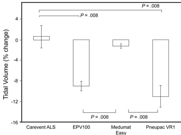
Fig. 2. Mean tidal volume variation over all the F<sub>IO<sub>2</sub></sub>, compliance, and resistance conditions, with the volume-cycled ventilators.
