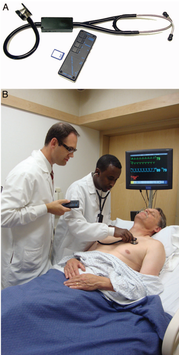
Fig. 7. A. Ventriroscope stethoscope and its transmitter and transceiver. B. Ventriroscope being used with a standardized patient.
