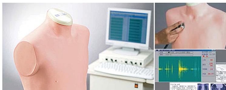
Fig. 2. Lung Sound Auscultation Skills and Training (LSAT) manikin and accompanying computer and auxiliary speakers. (Courtesy of Kyoto Kagaku.)
