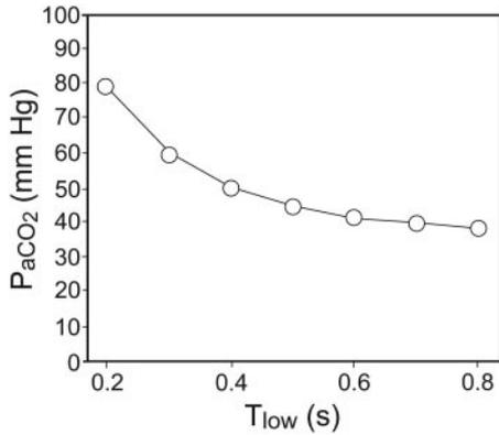
Fig. 6. This figure illustrates the dependence of simulated P<sub>aCO<sub>2</sub></sub> on the T<sub>low</sub> setting.
