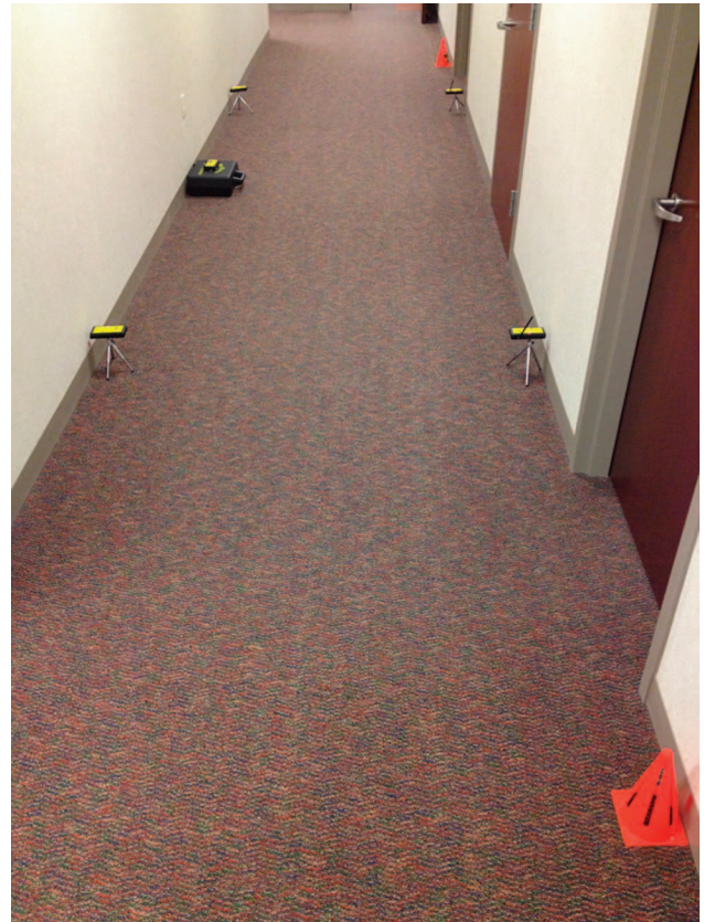
Fig. 2. Automated gait speed timing setup.
