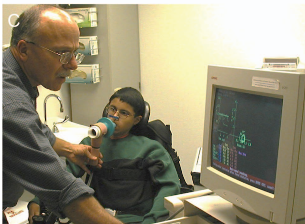
Fig. 1. Measuring cough peak flow. A: Asthma peak flow meter set up to measure peak cough flow with mask. B: Measuring cough peak flow with asthma peak flow meter and mask. C: Measuring cough peak flow with computerized spirometer. With permission. From Reference 32.
