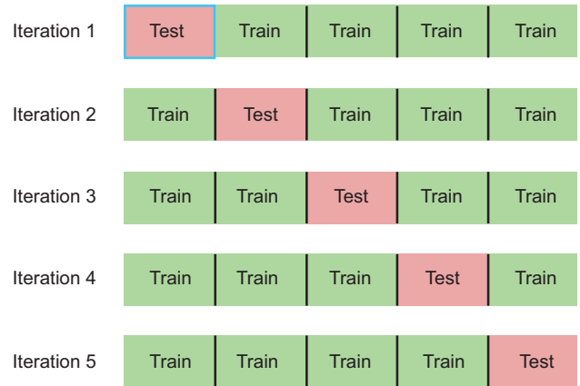
Fig. 1. Illustration of 5-fold cross-validation. In the first iteration, a portion of the data (one fifth of all cases) is assigned to testing, with the remaining data being available for training the machine learning model. In the second iteration, a different portion of the data (but still one fifth of all data) is assigned to testing. This process continues until all cases have been used for training and for testing. Summary statistics are compiled from each iteration, and the final results that are communicated in a paper reflect the average results from each iteration.
