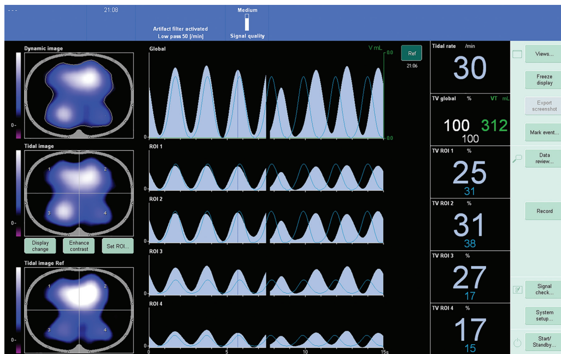
Fig. 3. The main display of a PulmoVista 500 device. The images on the left are also represented by waveform graphs in the center and percentage distribution on the right. The waveforms and percentage distribution are separate and represent the global and regional information. ROI = region of interest.
