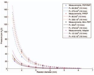
Fig. 2. Graph and calculated model of the pressures (P) from the different resistors according to resistor diameter (d). Solid lines show flow at 10 L/min, and dashed lines show flow at 18 L/min.
