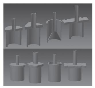
Fig. 1. Front views and cross-sections of the resistors tested. From left to right: Pep/Rmt system, Pipe P, Mini-PEP, and 15-mm endo-adapter.
