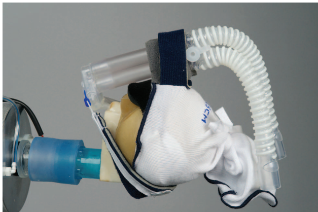
Fig. 1. Validated nasal model attached to the foam craft ball to construct a physical model with which a size 25–29-cm Fisher & Paykel bonnet would snugly fit.
