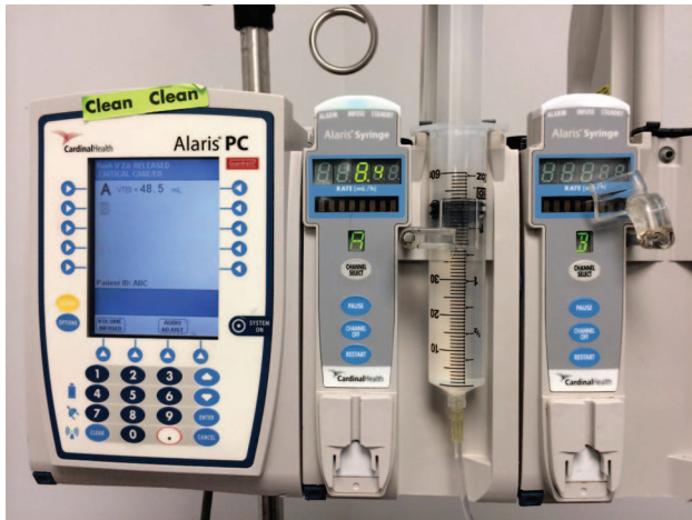
Fig. 6. Intravenous pump with 60-mL syringe.
