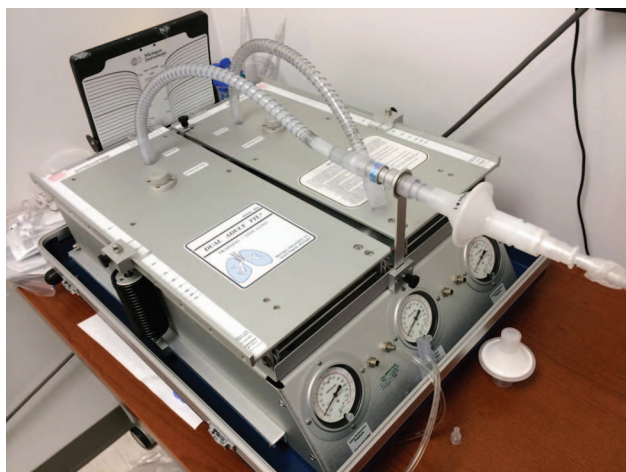
Fig. 1. Test lung, filter, and endotracheal tube.
