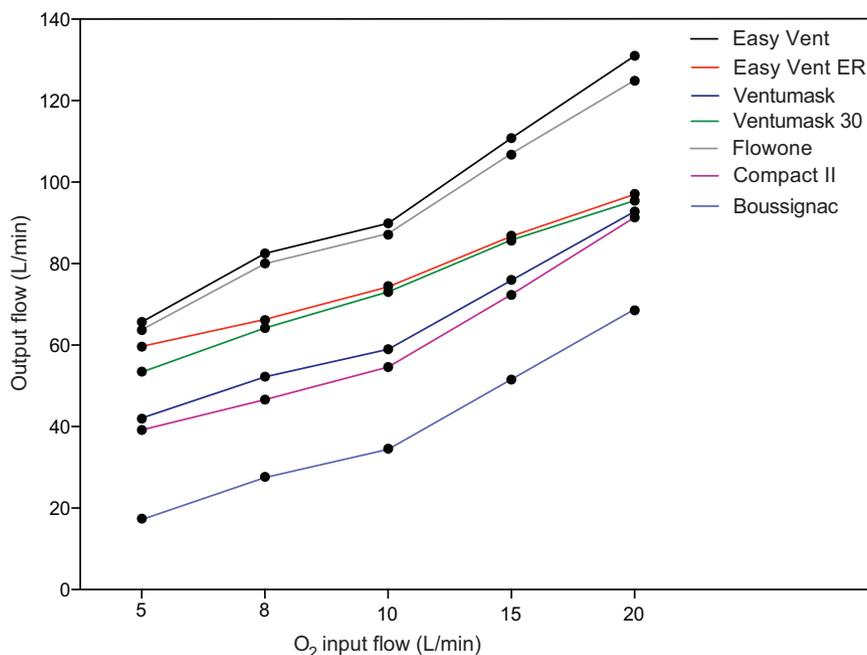
Fig. 1. Output flow generated by each device according to the O<sub>2</sub> input flow.
