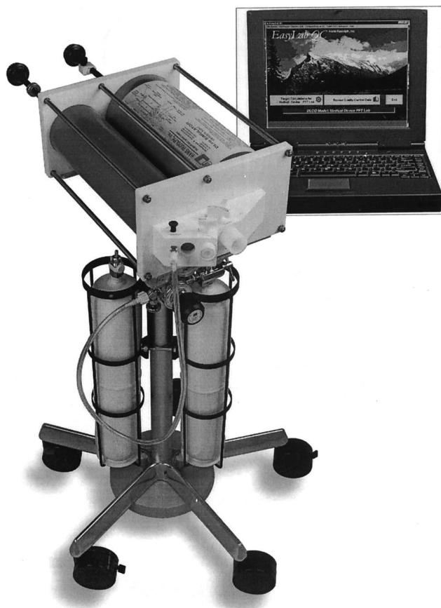
Fig. 2. A D_{LCO} simulator designed to test the accuracy of D_{LCO} measurement instruments. The simulator produces known volumes of precision gases that simulate human breath. The device can reliably simulate the same value to within fractions of a D_{LCO} unit (mm CO/min/mm Hg). (Courtesy Hans Rudolph Inc, Kansas City, Missouri)
