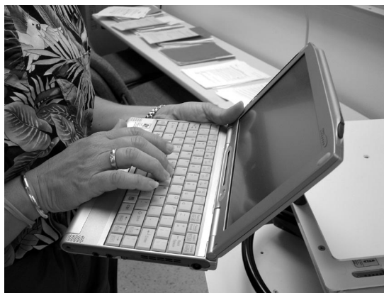
Fig. 1. Notebook computer (P-1120, Fujitsu, Santa Clara, California) with touch-screen and integrated wireless local-area-network capability. This is one of several options for mobile charting devices.
