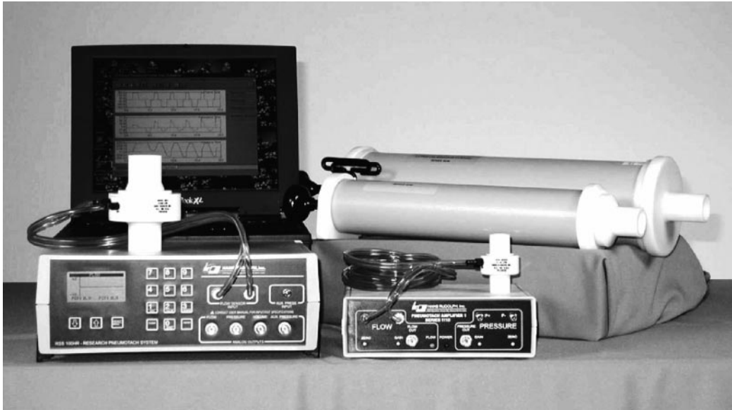
Fig. 4. Laboratory-grade, screen pneumotachometers with their signal-processing units and a display monitor. These units are available in various sizes to accommodate various sizes of animal or human subject. Similar configurations of these pressure-gradient devices are incorporated into many intensive-care ventilators. Note the 2 sizes of transducer shown, the larger one intended for adult patients and the smaller one for pediatric patients. (From Reference 5, with permission.)
