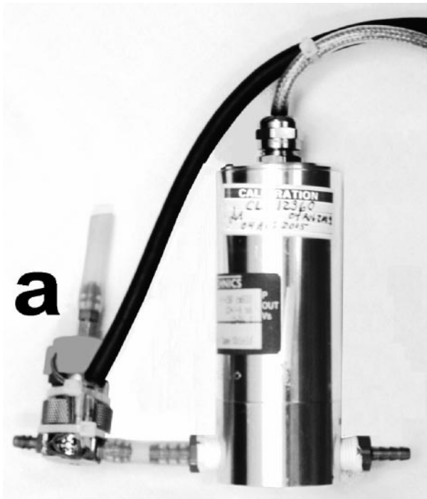
Fig. 3. Laboratory-grade pressure transducer. Note the calibration sticker on the cylinder. When combined with a 3-way solenoid valve (a), periodic activation of the valve (autozeroing) eliminates the drift error.
