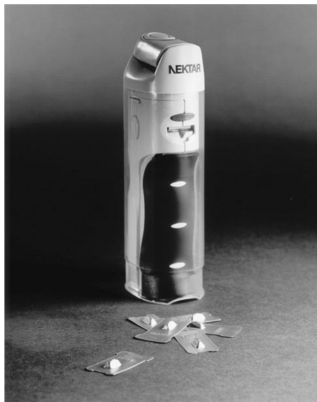
Fig. 5. Prototype of the Nektar PDS (“pulmonary delivery system”) for Exubera. The device slides open and closed like a telescope, for compact carrying and portability. The patient opens the device, inserts the foil blister (which contains the powdered medicine), and pumps the handle, which compresses a small amount of air inside the device. When the patient pushes the button, the compressed air is released at high velocity, which aerosolizes the powder and sends the aerosol into the chamber, where it is a stationary cloud. The patient then inhales the aerosol from the chamber. The patient receives the medicine first, followed by a volume of air, which helps push the drug deep into the lung. (Courtesy of Nektar Therapeutics.)
