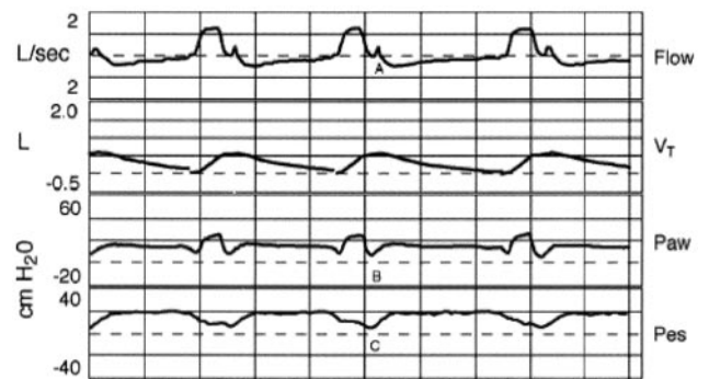
Fig. 4. Scalar waveforms taken from Patient 3 at a pre-set tidal volume ( V_T ) of 6 mL/kg revealed sustained inspiratory effort with a secondary low-level flow delivery from the ventilator during the end-inspiratory pause (A), resulting in an average ventilator-delivered V_T of 6.9 mL/kg. The Dräger E-2 ventilator has a backup algorithm that controls airway pressure ( P_{aw} ), even during volume-control ventilation. One of these algorithms allows the high-pressure servo valve to open if the P_{aw} falls -0.2 cm H 2 O below baseline [personal communication, Dräger Medical]. A drop in P_{aw} below baseline was evident during the end-inspiratory pause on each breath (B), as was continued patient effort into the inspiratory pause (C). P_{es} = esophageal pressure.
