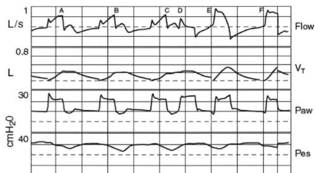
Fig. 6. Scalar waveforms of gas flow, tidal volume ( V_T ), airway pressure ( P_{aw} ), and esophageal pressure ( P_{es} ) taken from Patient 13 during pressure-control ventilation. This figure represents a common finding whereby chest-wall stiffening at the onset of a mechanical breath results in an initially low ventilator flow delivery that begins to taper off. When the patient's inspiratory effort begins later in the inspiratory phase, the resulting ventilator flow paradoxically becomes ascending, and inspiratory effort continues into the expiratory phase (breaths A and B). The same phenomenon occurs during breath C, which results in a double-triggered breath (D). Breaths E and F represent conventional patient-triggered breaths whereby the ventilator flow pattern changes according to the intensity of inspiratory effort.
