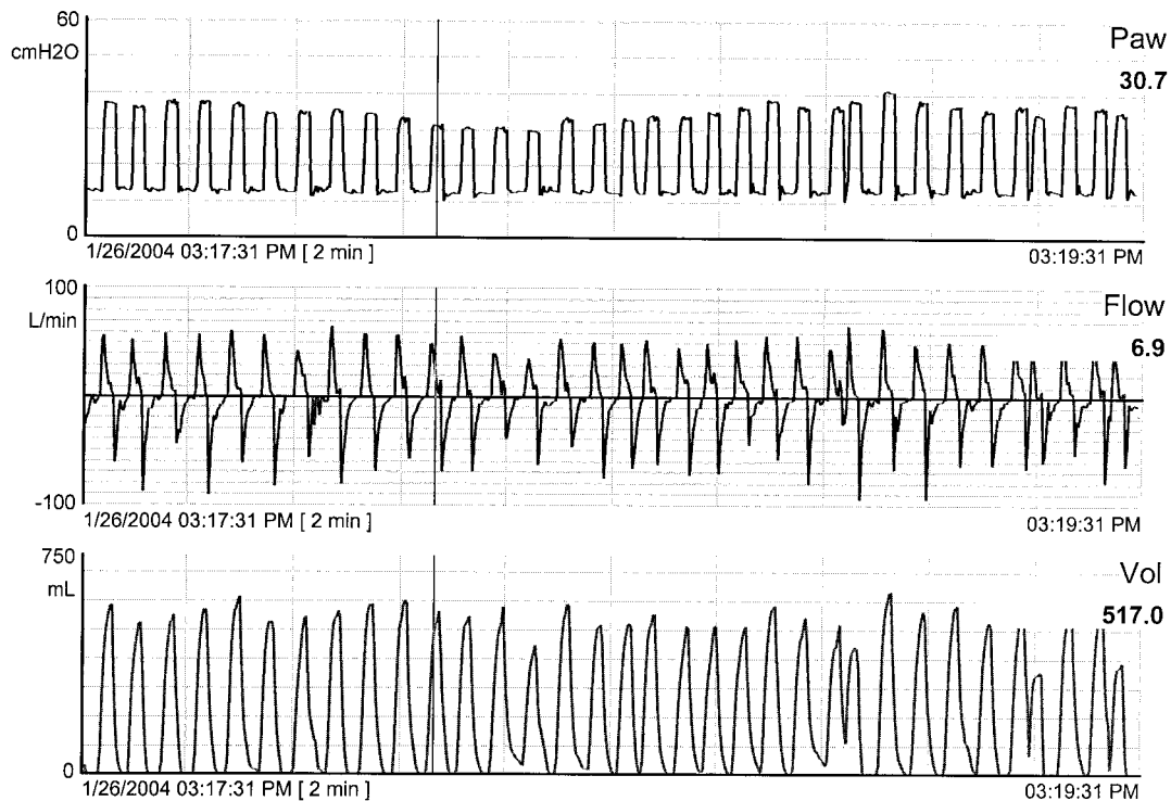
Fig. 20. Airway pressure ( P_{aw} ), flow, and volume waveforms demonstrating the response of a dual-control algorithm over a 2-min period with varying patient effort. The tidal volume varies above and below the target (500 mL) by as much as 150 mL. In our experience this is a common occurrence during dual-control ventilation with an active patient (see text).
