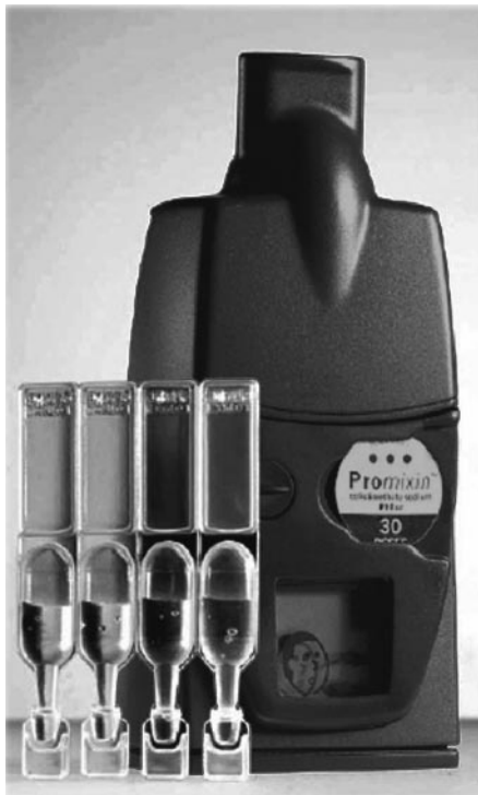
Fig. 9. The I-Neb adaptive aerosol delivery system offers 2 breathing patterns. It is the first handheld device that regulates the pattern of breathing.
