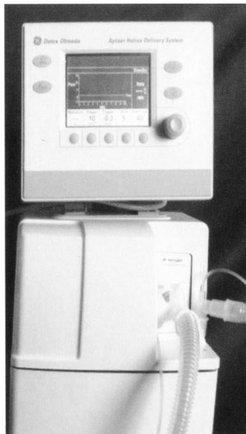
Fig. 2. The Aptair heliox system delivers heliox from an H-size cylinder, and provides spontaneous, monitored, noninvasive pressure support, with alarm settings, via face mask.
