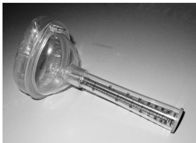
Fig. 4. Peak-cough-flow meter with an air-cushion face mask.
