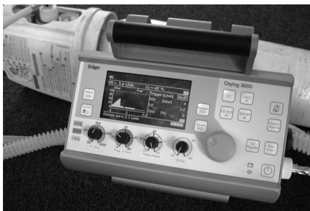
Fig. 1. The Oxylog 3000 transport ventilator. The user interface facilitates direct and rapid access to the main ventilation parameters via dials similar to those found on simple pneumatic ventilators (eg, tidal volume, respiratory rate, maximum inspiratory pressure, and fraction of inspired oxygen). Advanced setting options can be selected by using the pressure-sensitive keys (for start-up procedure or ventilation mode, for example) and the master click-dial. VC = ventilation contrôlée (controlled ventilation). This also allows access to the assist-control ventilation mode when the inspiratory trigger is activated by the master click-dial. VACI-AI = ventilation assistée contrôlée intermittente - aide inspiratoire (synchronized intermittent mandatory ventilation - pressure-support ventilation). VS PEP-AI = ventilation spontanée avec PEP - aide inspiratoire (spontaneous ventilation with positive end-expiratory pressure - pressure-support ventilation). BIPAP-AI = biphasic positive airway pressure (Dräger-specific ventilation mode) (pressure-support ventilation). The BIPAP-AI mode was not tested in the present study.
