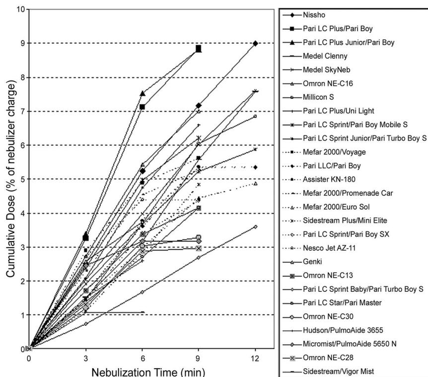
Fig. 4. Budesonide mass collected on inhalation filter (percentage of nebulizer charge) of budesonide inhalation suspension over 3-min intervals during infant breathing patterns for up to 12 min of nebulization. The slope of each curve represents the rate of budesonide delivery.
