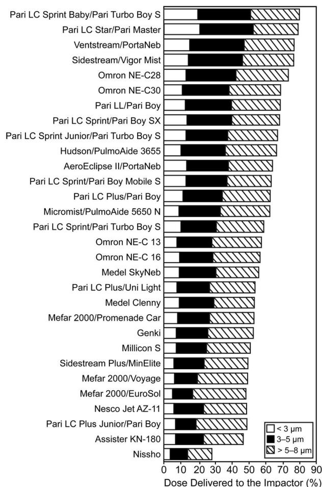
Fig. 2. Droplet size distribution of budesonide inhalation suspension up to 8 μm diameter (mean of 3 tested units), expressed as a percentage of budesonide mass delivered to the impactor.
