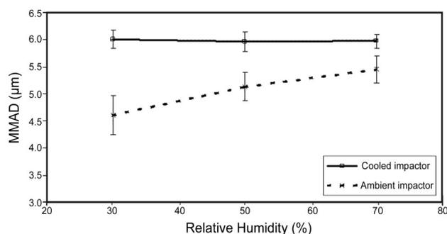
Fig. 1. Mass median aerodynamic diameter (MMAD) as function of relative humidity, of budesonide inhalation suspension nebulized with a jet nebulizer.
