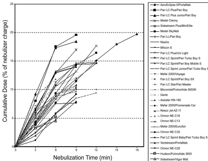
Fig. 5. Budesonide mass collected on inhalation filter (percentage of nebulizer charge) of budesonide inhalation suspension over 3-min intervals during child breathing patterns for up to 18 min of nebulization. The slope of each curve represents the rate of budesonide delivery.
