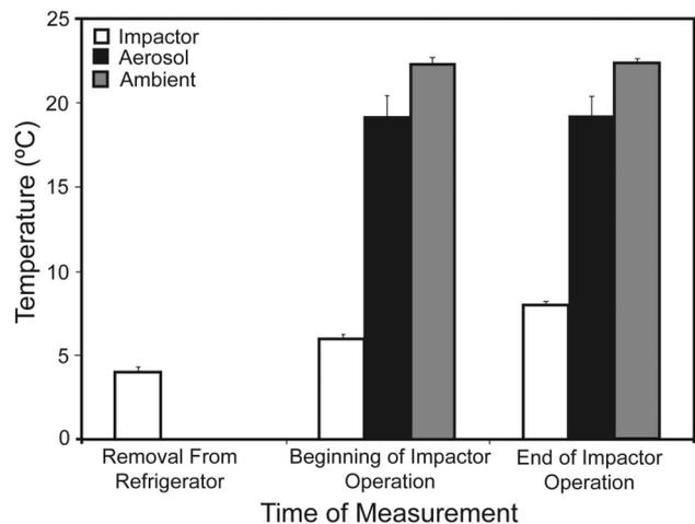
Fig. 3. Impactor and aerosol temperature.
