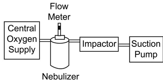
Fig. 2. Experimental setup to measure aerosol particle size.
