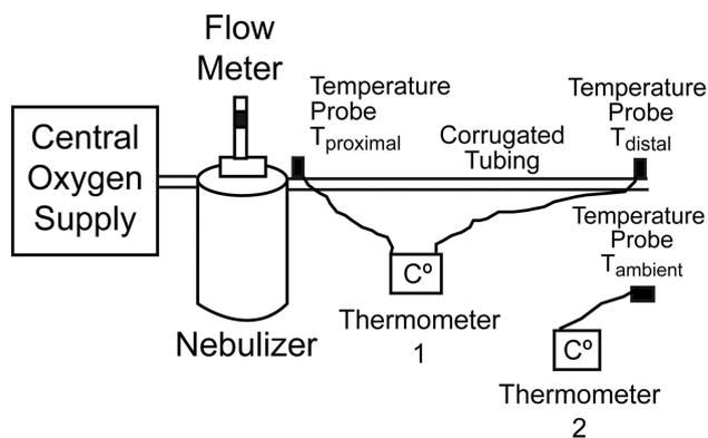
Fig. 4. Experimental setup to measure aerosol temperature and tubing retention.
