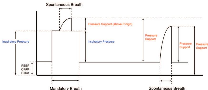
Fig. 1. Idealized airway pressure waveform, showing various conventions used for pressure parameters (see Table 1). Note that there are 2 ways to define the inspiratory pressure (blue) of a mandatory breath, and 4 ways to define the pressure support of a spontaneous breath (red). PEEP = positive end-expiratory pressure. CPAP = continuous positive airway pressure. P-low = low pressure.
