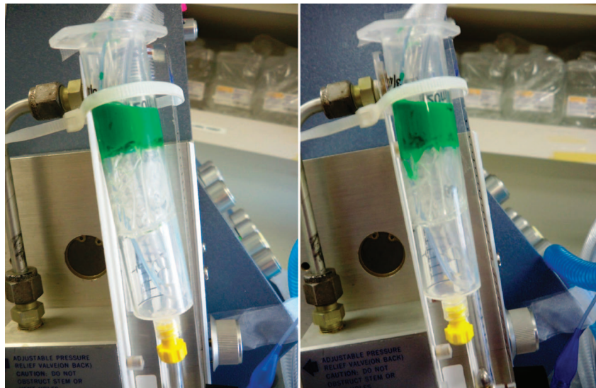
Fig. 1. Left: Mallinckrodt 7.5-mm inner-diameter endotracheal tube with a lubricated PVC cuff, 2 hours after 3 mL of colored whole milk was instilled above the cuff and the model was mechanically ventilated at 5 cm H 2 O PEEP and 5 cm H 2 O inspiratory pressure (ie, pressure below the cuff). Immediately after taking this picture, I agitated the cuff by moving the endotracheal tube up and down and side to side. Right: Three hours later (2 hours after agitating the cuff plus 1 hour after disconnecting the ventilator and thus removing the positive pressure below the cuff).
