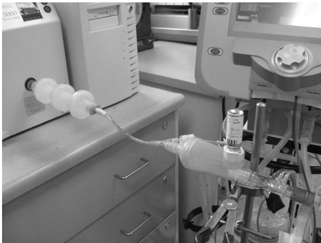
Fig. 2. Simulated aerosol delivery with the AeroChamber Mini valved holding chamber (VHC) during mechanical ventilation. A: Schematic. B: Setup with aerosol-collection filters at the distal end of the endotracheal tube (ETT). pMDI = pressurized metered-dose inhaler.
