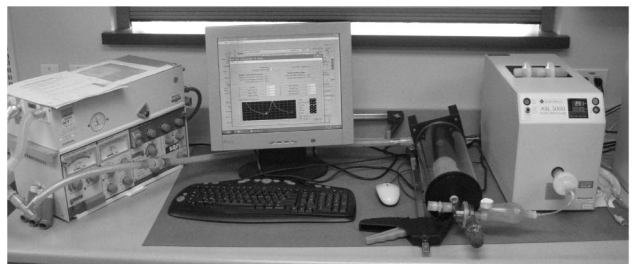
Fig. 3. Simulated aerosol delivery with the AeroChamber Mini valved holding chamber (VHC) during manual resuscitation. A: Schematic. The servo ventilator drives the resuscitation bag in an airtight plethysmograph-type chamber to provide a consistent, reproducible breathing pattern via the VHC and endotracheal tube (ETT). B: Setup with airtight chamber for manual resuscitation bag. pMDI = pressurized metered-dose inhaler.
