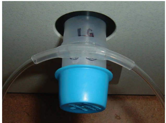
Fig. 2. Model nares, made from a 22-mm inner-diameter adapter, with nasal cannula in place, attached to the lung simulator. The cap on the distal end of the adapter prevents leak, which simulates a closed-mouth scenario. LG = large (ie, the large nasal prongs indicated in Fig. 1).
