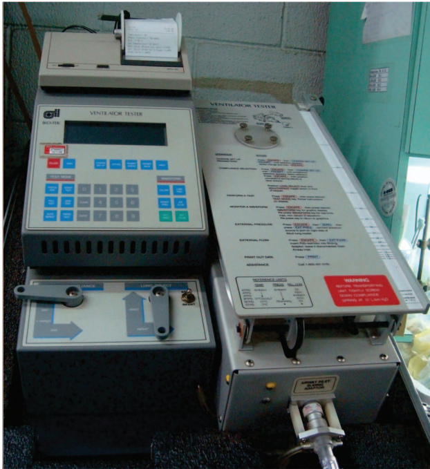
Fig. 1. Test lung model and ventilator tester.
