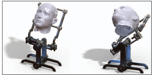
Fig. 2. Illustration of the mannequin setup for the vertical and horizontal movement evaluations. The platform uses gear motors and encoders to pivot the mannequin head in 2 dimensions. Control for the motors is via a Labview interface.
