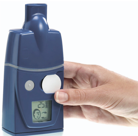
Fig. 6. I-neb adaptive aerosol delivery system. This delivery system generates aerosol using vibrating mesh technology. Metering chambers control the drug dose, delivering a preset volume ranging from 0.25 to 1.4 mL, with a residual of ~0.1 mL. Medication is delivered into 50–80% of each inspiration based on a rolling average of the last 3 breaths. Courtesy Philips Respironics.
