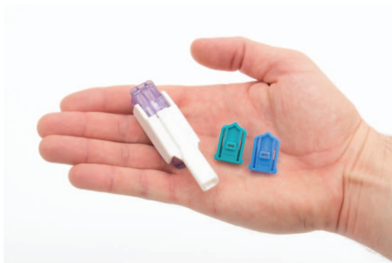
Fig. 9. The Afrezza, a second-generation device for delivering insulin. It is a pocket-size drug-device combination product. Insulin microparticles (Technospheres) are introduced into the device in an aspirin-like tablet, which is crushed when the device is closed, releasing drug as a dry powder. Courtesy MannKind.
