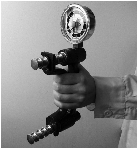
Fig. 2. The hydraulic gauge for hand-grip force, measurement in kg.
