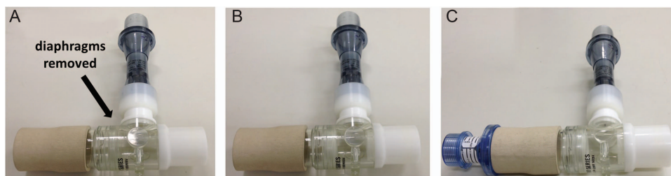
Fig. 1. Experimental device applied to obtain different EPAP intensities during exercise. A: Without EPAP, B: EPAP 5 cm H 2 O, and C: EPAP 10 cm H 2 O. EPAP = expiratory positive airway pressure.
