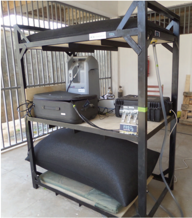
Fig. 1. Low-pressure oxygen storage system installed in Mbarara, Uganda. The lower bag is inflated with stored oxygen, whereas the upper bag is holding the water ballast.
