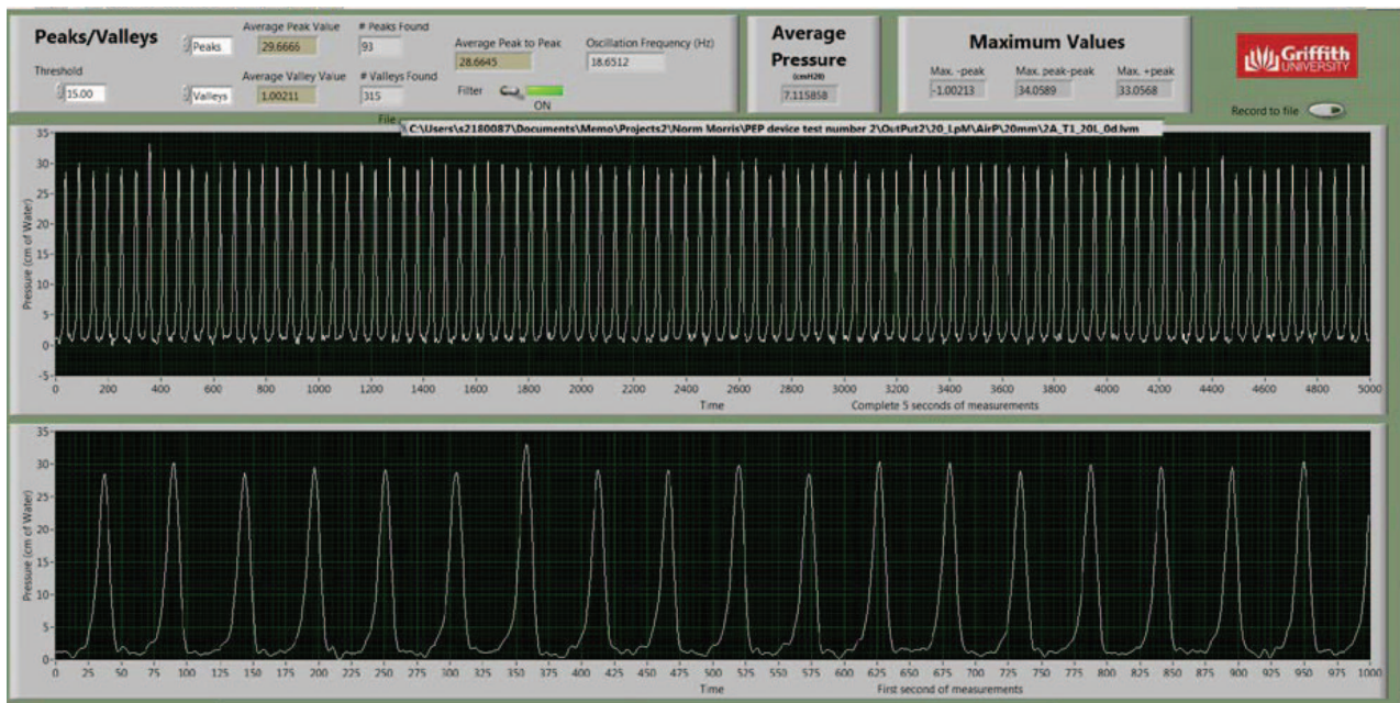
Fig. 2. Trial figure for the Flutter device at an inclination angle of 0^{\circ} and 20 L/min flow.
