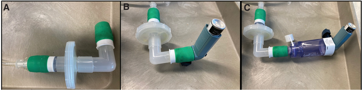
Fig. 1. Recovery apparatus. A: Recovery apparatus alone; B: recovery apparatus with pMDI attached; and C: recovery apparatus with pMDI and valved holding chamber attached.
